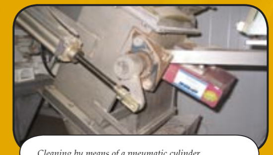
Cleaning by means of a pneumatic cylinder.
