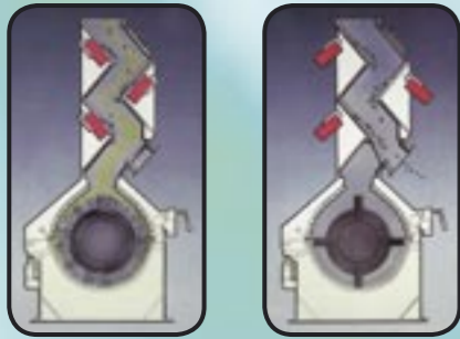
Left: cascade magnet in operation.
