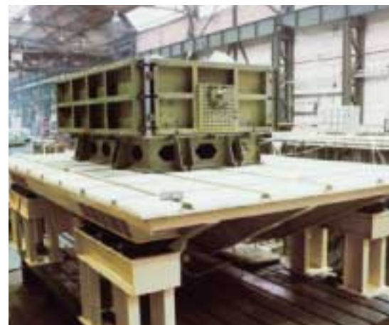
Vibrating tables with continuously adjustable magnetic vibrators ensure perfect material compaction in production and during packing
