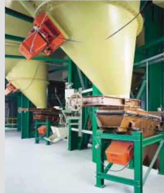
Continuous charging of ingredients for glass manufacture with feeding into the melting end takes place with finely controlled conveyor troughs with maintenance-free magnetic drives. Additional impact vibrators on the bunker walls prevent the material from caking to the sides and from forming bridges
